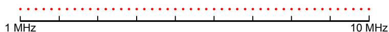
Figure 6-21: Linear x-axis scaling: the distance between the sweep points is equal, e.g. 200 kHz
